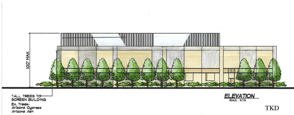
Typical Screening of Large Buildings
