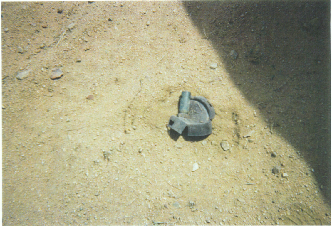
J-5 Remnant of spotting charge used in M38A2 practice bomb - discovered on southern boundary of site.
