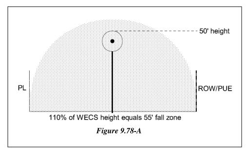
**Height.** The vertical distance from ground level to the top of the WECS, including the blade when at its highest point.
