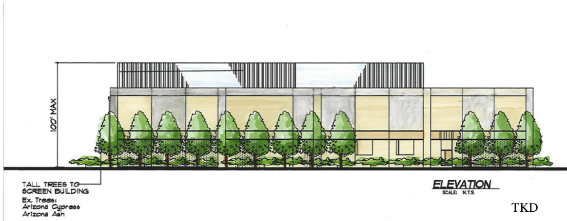
Typical Screening of Large Buildings
