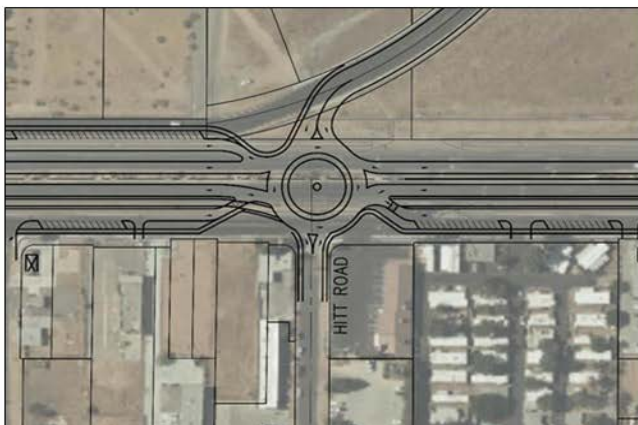
In both Alternatives 1 and 2, the realignment of Headquarters Drive to intersection Highway 18 across from Hitt Road improves access to the land north of Highway 18, provides a new connection between the north and south sides of Highway 18, and most importantly, it dramatically shortens the nearly ½-mile stretch of Highway 18 without a pedestrian crossing.
