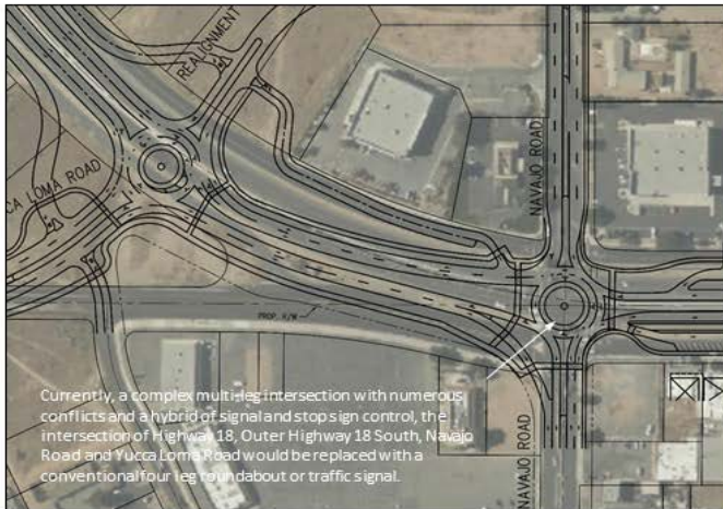
In Alternative 1, the realignment of Yucca Loma Road to Highway 18 eliminates the existing six leg intersection of SR 18 / Outer Highway 18 South / Navajo Road / Yucca Loma Road and replaces it with a multi-lane roundabout.
