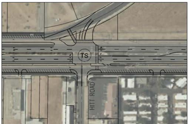
In both Alternatives 1 and 2, the realignment of Headquarters Drive to intersection Highway 18 across from Hitt Road improves access to the land north of Highway 18, provides a new connection between the north and south sides of Highway 18, and most importantly, it dramatically shortens the nearly ½-mile stretch of Highway 18 without a pedestrian crossing.
