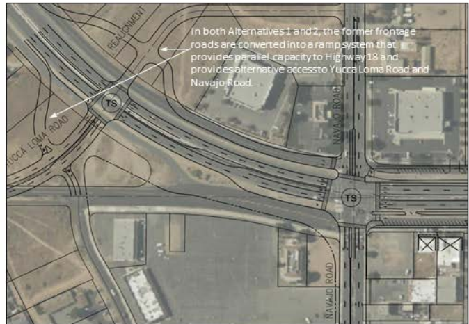
In Alternative 2, the realignment of Yucca Loma Road to Highway 18 simplifies the existing six leg intersection of SR 18 / Outer Highway 18 South / Navajo Road / Yucca Loma Road and replaces it with a conventional four leg signalized intersection.
